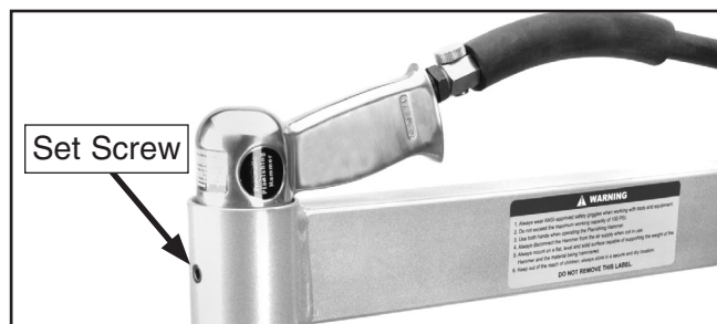
Figure 7. Hammer installed in C-frame.
